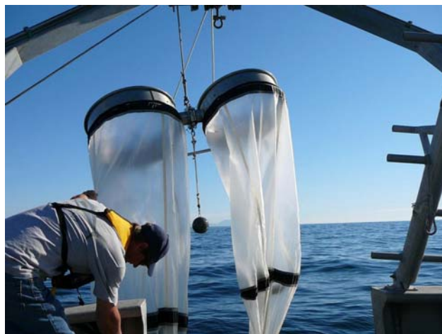
Figure 2-2. Paired plankton nets used for sampling (Tenera, 2010)
