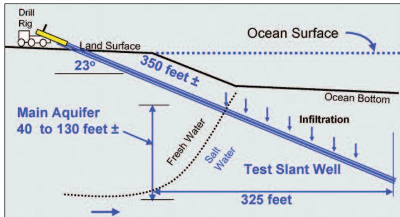
Slant Wells are a type of sub-seafloor system that draws seawater from beneath the seafloor.
