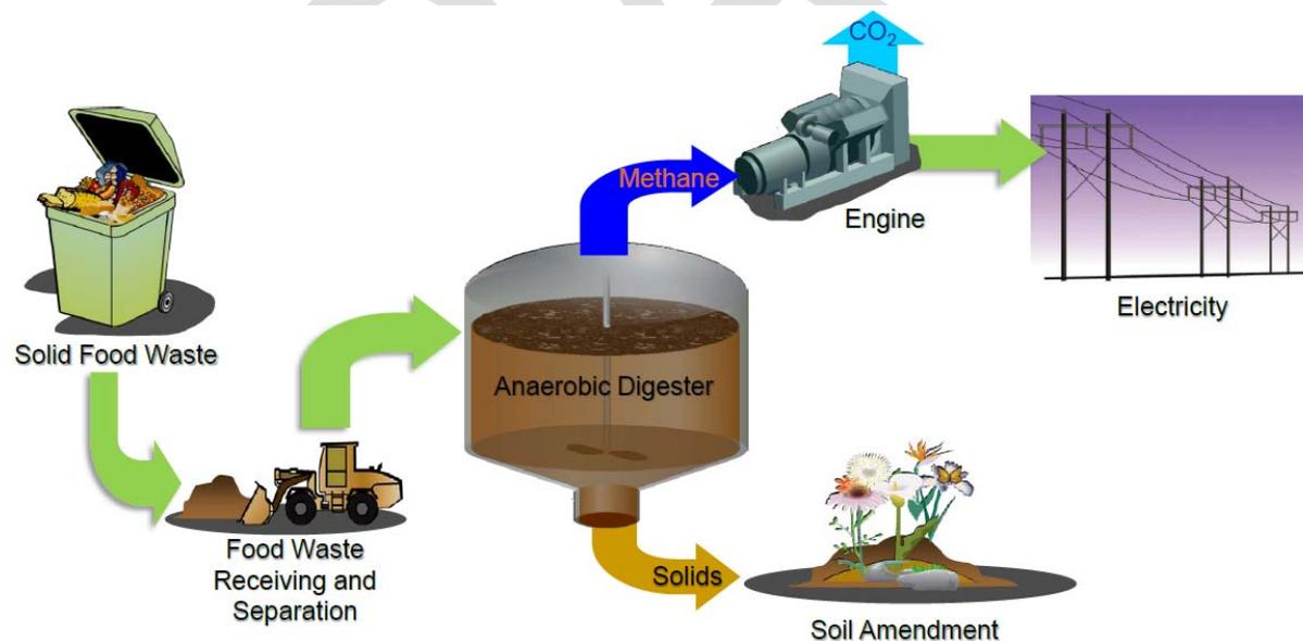
A combustion generator operating on digester gas produces emissions, including CO<sub>2</sub> and a small amount of other gases. However, these emissions are not accounted for as “GHG emissions” because they come from a non-fossil fuel source and are considered biogenic. The combustion generator process converts the more potent GHG (methane) to less potent GHG (carbon dioxide) while extracting energy in the process. The emissions of CO<sub>2</sub> (and a small
